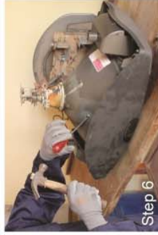
Fa "screw driver" to daɛɛɛ akataso no so. Tue tube no ha kakra kopem se wobete se mfrana Ere-ba
